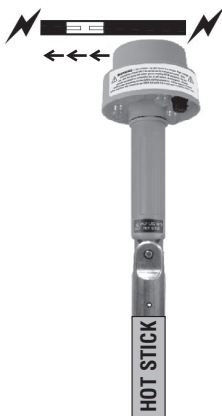
Fig. 2: Finding a cable fault
